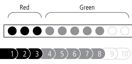
**Note:** If ten Indicator light segments are illuminated, the output voltage may be more than 10 kV (10,000 V).
